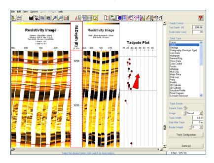
enhancing the quality of the data. These include speed corrections, pad and pad/flap correlations, swing-arm, EMEX and gain correction and "dead" button removal. Individual button shifts can also be applied.
