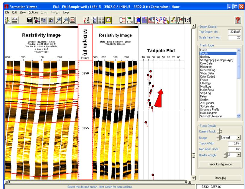
The data can be displayed in the false color image mode or as individual wiggle traces. In addition a 'core-like' display of the imaging data can be displayed. This can be viewed from any angle or direction.
